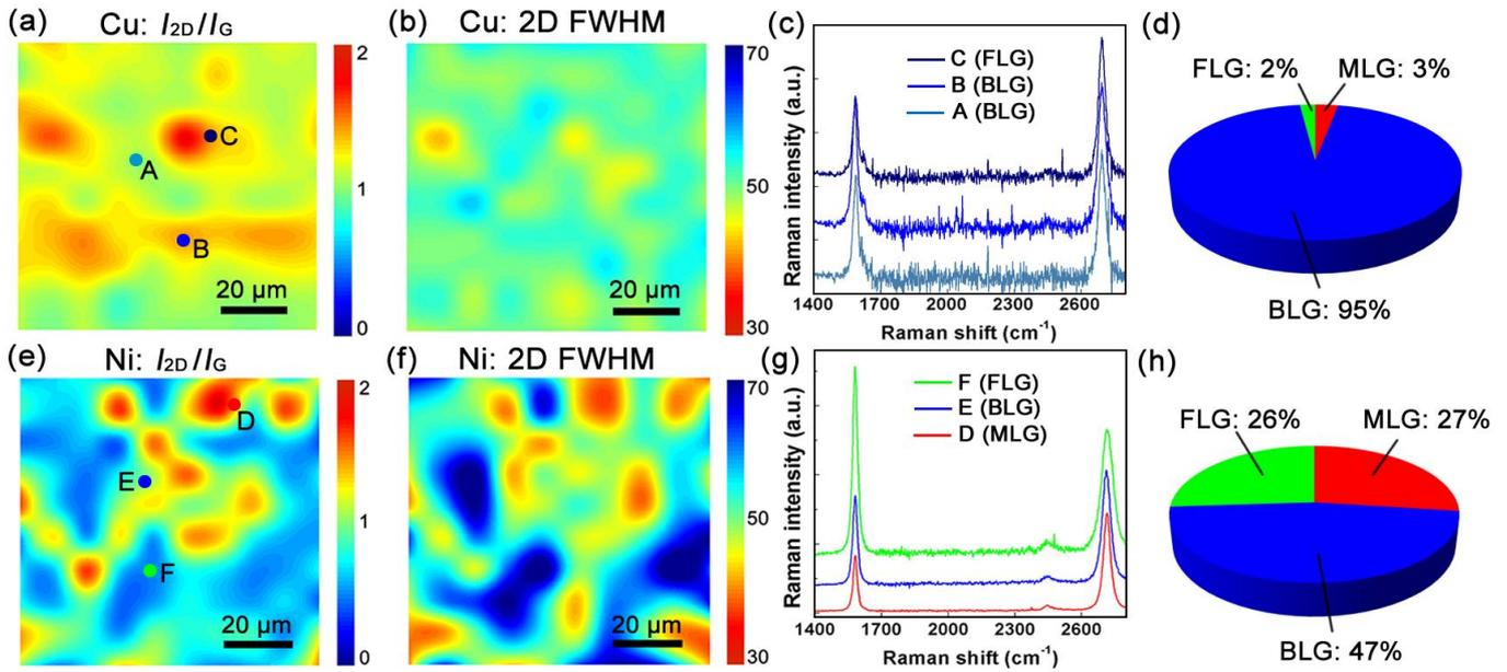
Fig. 2: Raman spectroscopic analyses of as grown graphene after transferred on Si/SiO<sub>2</sub> substrates. Raman maps of  $I_{2D}/I_G$  and 2D FWHM of graphene grown on (a, b) Cu and (e, f) Ni. (c, g) Raman spectra of three corresponding points in (a, e). The percentages of MLG, BLG and FLG graphene grown on (d) Cu and (h) Ni.
