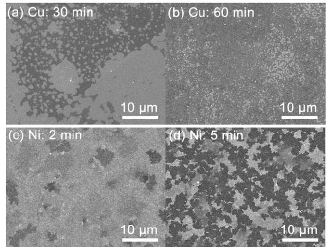
Fig. 1: SEM images of graphene with different morphologies grown on (a, b) Cu and (c, d) Ni substrates.
